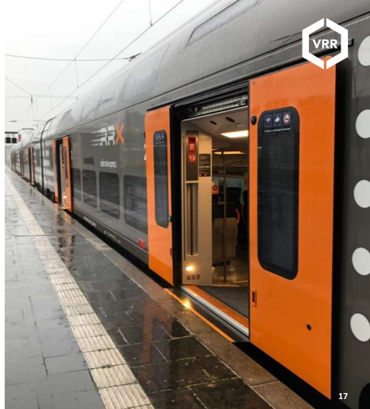
Double-deck coach with an average clear width of the outer door of 1800 mm
